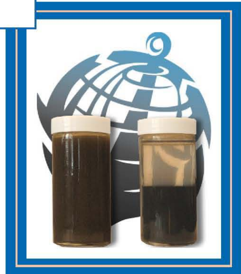
Influent Sludge from the Treatment Device (left); Thickened, Reacted Sludge Ready for Decant (right)
